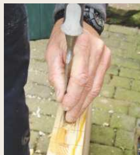
▲ Pic.3 ...which was then cleaned up with a chisel
